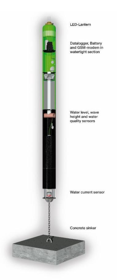
*Figure 4. Schematic figure of SmartBuoy system. Sea trials utilizes water quality monitoring option, but the system can be used simultaneously also for water level, current and wave height monitoring.*
