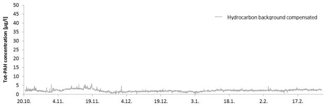
Figure 8. Collected hydrocarbon data processed with initial calibration. The data will be re-calibrated when more reference data is available.
